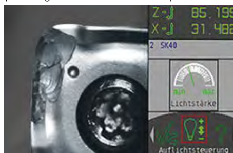
Cutting edge inspection – 12-fold magnification of the cutting edge in incident light for quality control (option)
