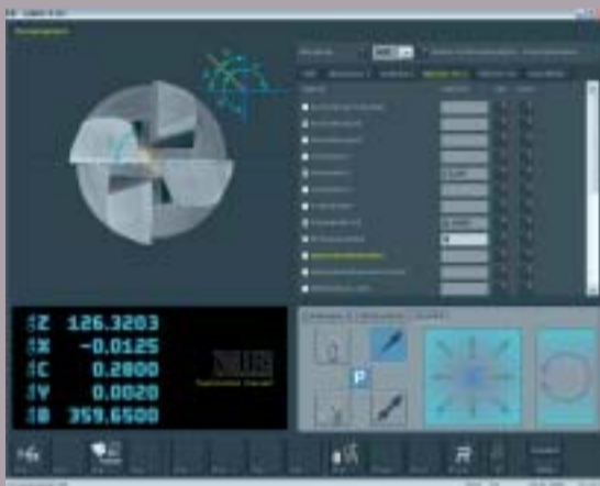
Select menu for measuring at the end: Example: chisel edge angle
