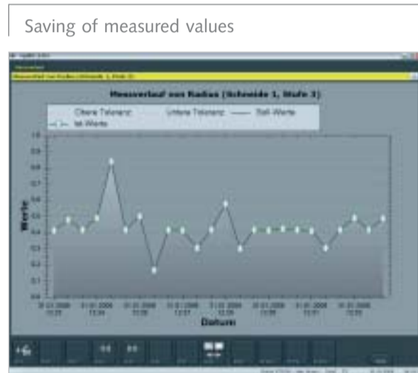
The measured values of saved tools are recorded automatically with each measurement, can be evaluated statistically and called up at any time.
