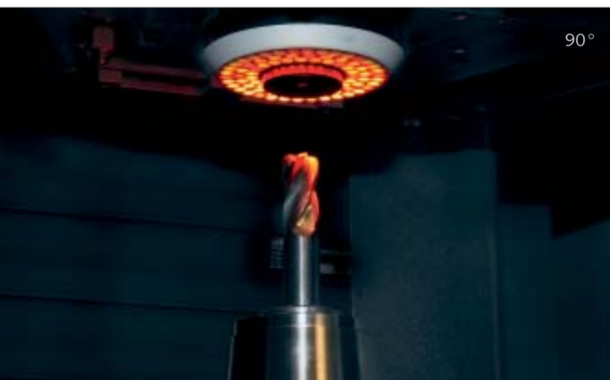
Axial, backlash-free positioning for automatic measurement of the end contour of tools.
