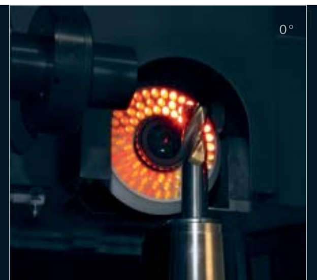
Radial, backlash-free positioning for automatically measuring the tools at circumference and in the chip space.
