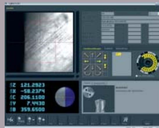
»expert« interactive configuration wizard: Example: effective cutting angle/illumination
