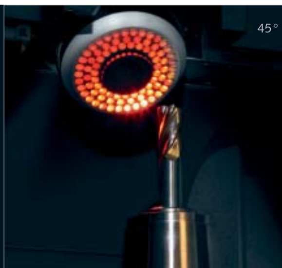
CNC-driven pivot position as required for measuring transition radii and slopes, for example of the edge honing.
