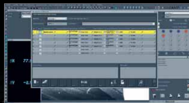
The measured wear features are transmitted control-specifically to the respective grinding machine at the push of a button.
