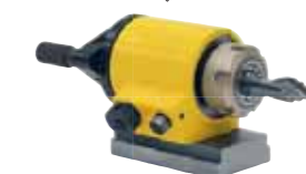
»pomRoto« rotation unit* clampable shank diameter as a result of collet chuck: 1.5 – 16 mm, max. tool length: 400 mm, rotation accuracy: 0.006 mm
